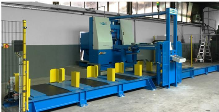
In the past few days the time arrived for our new band saw system to go on stream. It has a feeding facility and an automated separating system for sorting the cut starting material and waste material. The band saw system is controlled by a Siemens S 7-1500 system. This investment has led to
